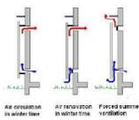
the top is opened to vent the hot air to the outside. Such venting makes the Trombe wall act as a solar chimney pumping fresh air through the house during the day, even if there is no breeze.
